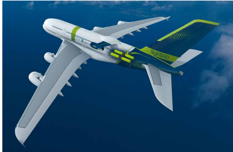
Hydrogen tanks in the future A380 ZEROe flight test demonstrator
