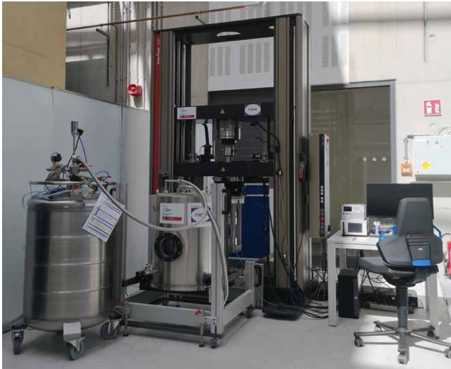
Tensile measuring machine for measurements in liquid nitrogen at -196°C at Bremen Fibre Institute
